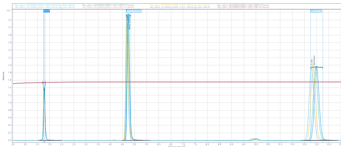
Annex 3: Chromatogram showing DAD and pressure profile of four injection of a test solution: uracil (0.02mg/ml), Methyl benzoate (0.7uL/mL), Naphthalene (0.24mg/mL). Flow: 0.2ml/min, Detection: 254nm, injection volume: 2µl, 155bar, Eluent: ACN/Water (60/40)
